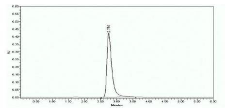
Figure 2. Typical Chromatogram for Cefotetan
